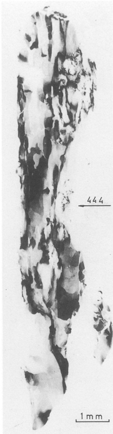
Figure 4 Topography of a wafer of ingot 2—growth speed: 2.4 \text{ cm day}^{-1} ; thermal treatment: T = 500^\circ\text{C} , t = 10 days.
